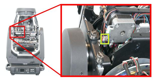
3. Optional. This step may be performed to help improve access to the gobo wheel module. On the prism module, find the 4-pin connector (denoted by the yellow box, above right) in the that is located behind the left-most electric motor, just beside the thumb screw on the left hand side of the prism module. Disconnect this connector.
